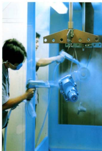
涂装流水线 EKB Coating Line
