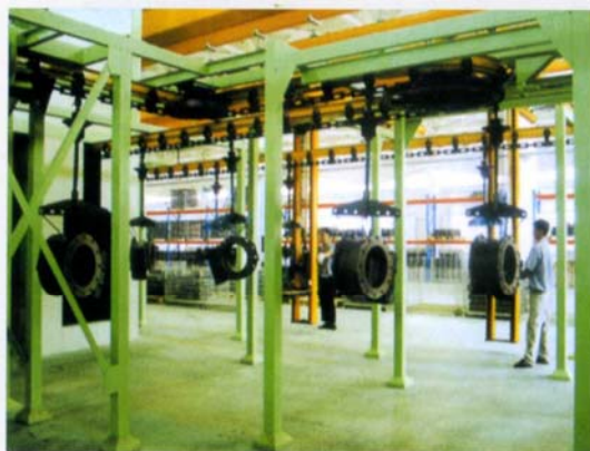
产品在流水线上喷丸后过程中 Products on the Blasting Line
