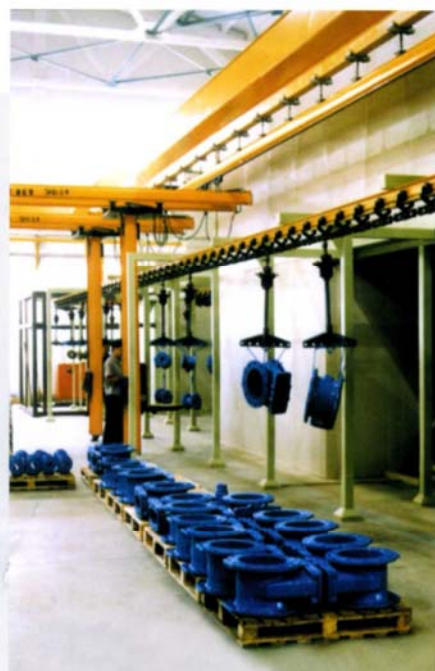
静电环氧树脂粉末涂装 Electrostatic Epoxy Resin Powder Coating
