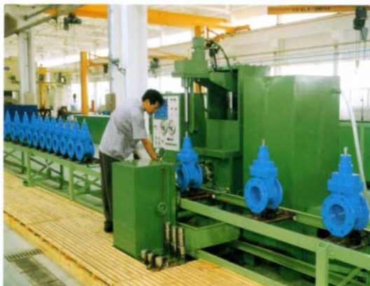
闸阀试验生产线 Gate Valves on the Testing Line
