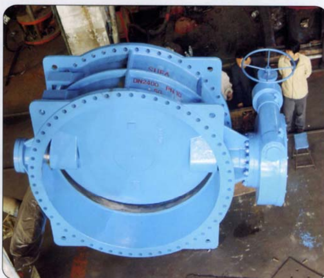
DN2400 手动蝶阀在出厂前作最后调试 Butterfly Valves with Handle wheel are Tested before ex-work
